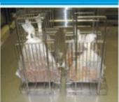
Place cooking rack into the base rack of the Rethermalizer. NOTE: Only one bag per cooking rack.
